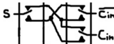
Since the carry-in and carry-in-negative levers move together, no pathway exists that allows them to touch and inadvertently energize each other. So, the optimization is okay in this case.
